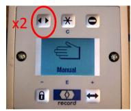
Pressing the hold open button twice puts the door to Manual Operation
